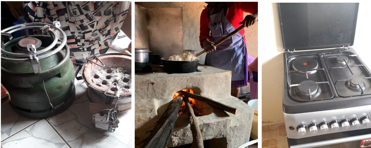
24 Figure S2. Typical stoves encountered in the study, with the LPG and charcoal stoves shown at left (with SUMs installed), 25 a traditional Chepkube stove at center, and a 4-burner LPG stove at right. 26 27
