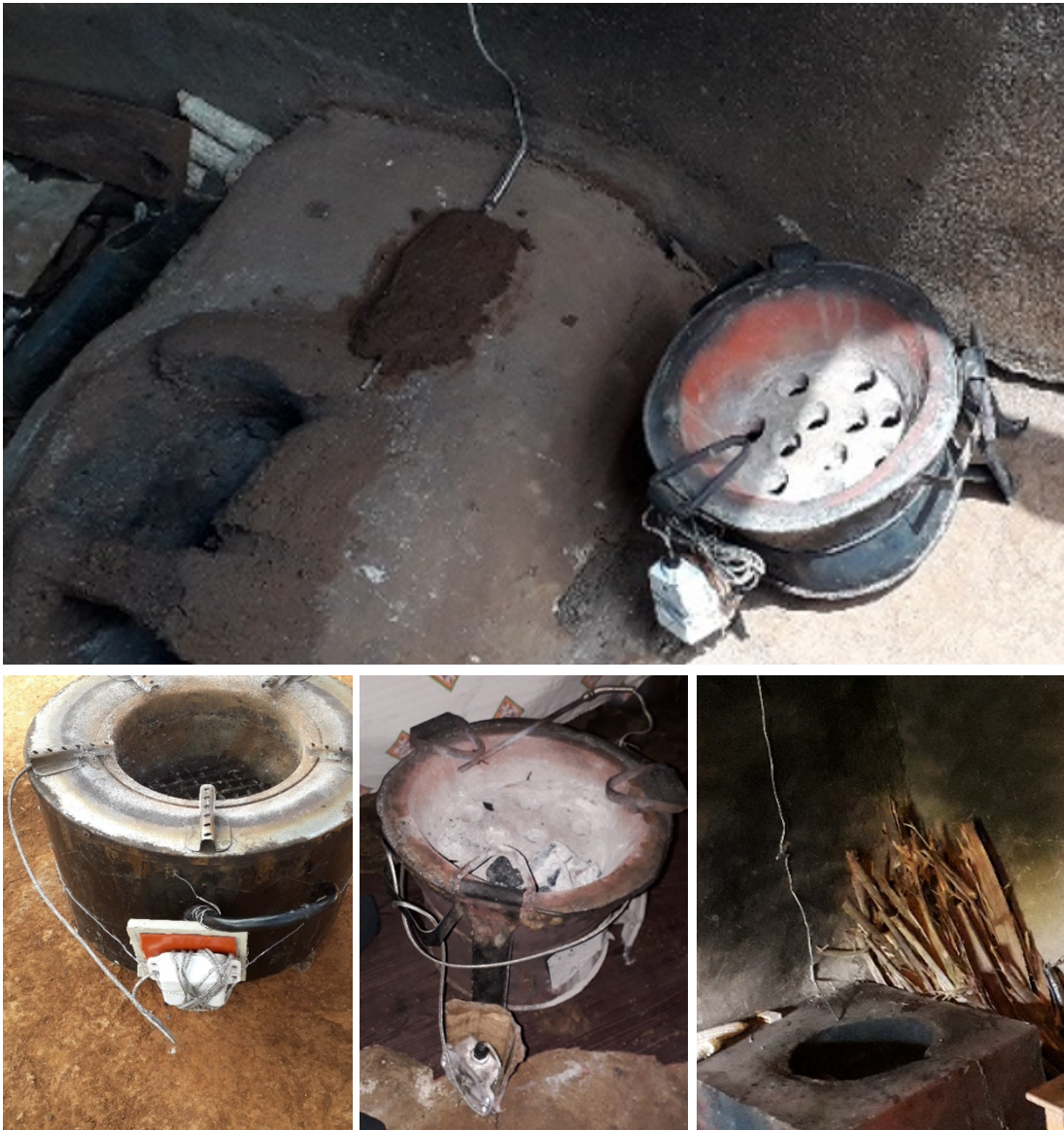
110 Figure S8. Photos showing SUMs installation on various stove types. On the portable stoves, the logger can be observed 111 affixed to the stove body, while on stationary stoves, the thermocouple is shown threaded to the zone of combustion.
