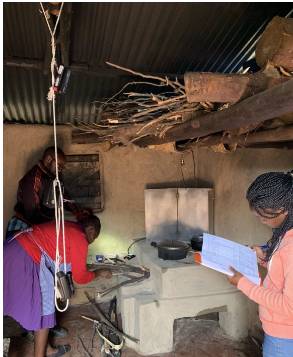
Figure S3. The emissions measurement system set-up to measure an LPG cooking event at left, and a biomass cooking event on a Chepkube stove at right. Note the stratified instruments hanging in the room as part of an intensive sample.
