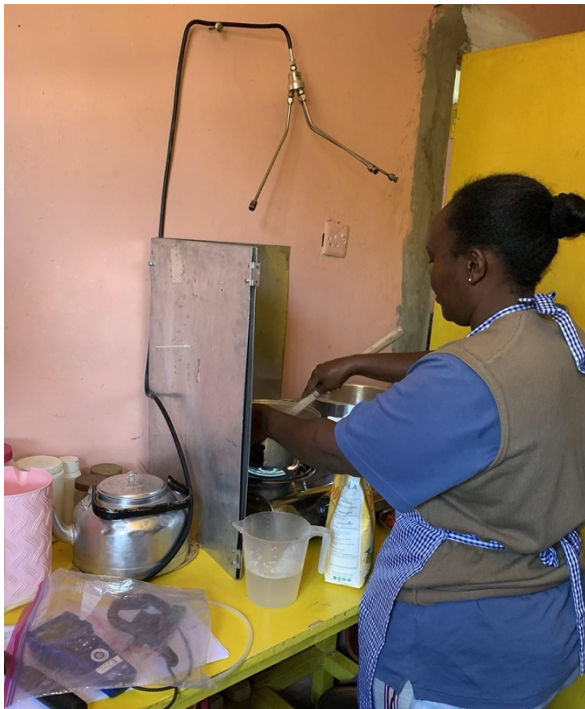
Figure S3. The emissions measurement system set-up to measure an LPG cooking event at left, and a biomass cooking event on a Chepkube stove at right. Note the stratified instruments hanging in the room as part of an intensive sample.
