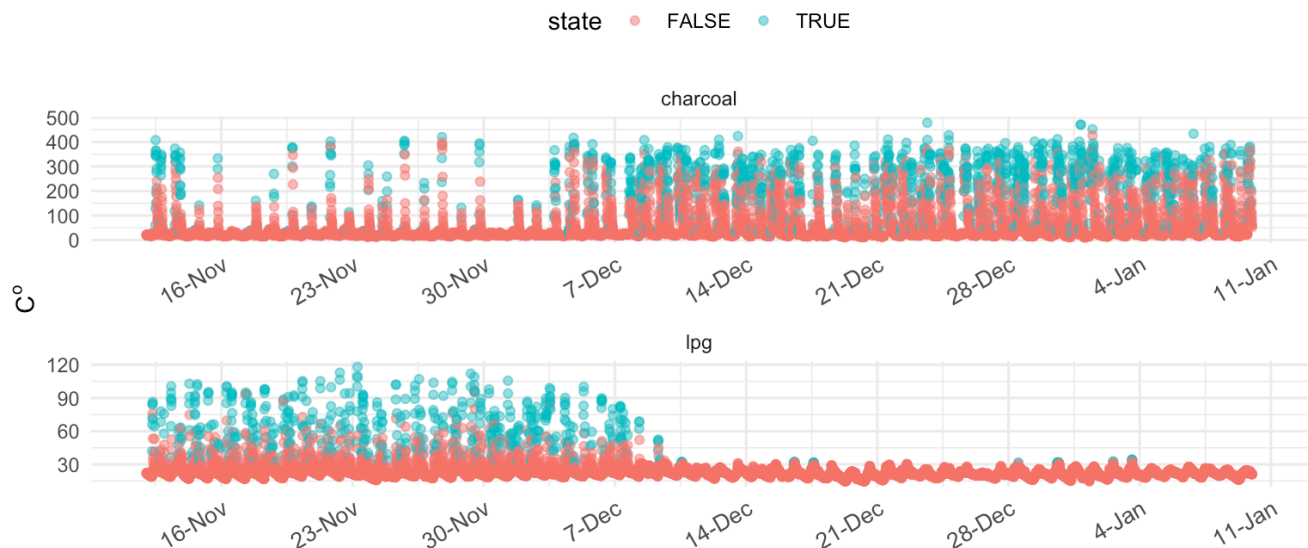
99 Figure S7. A typical temperature trace for a single home, showing the diurnal temperature trends typical in SUMs 100 measurements, and the peaks produced by cooking events on two different stoves. TRUE indicates points identified as 101 cooking, while FALSE indicates not-cooking periods.
